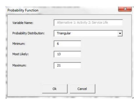
RealCost – Service Life for SMA and HMA Pavement Rehabilitation 2034 and 2047 (Alternative 1: Activities 2 and 3)
