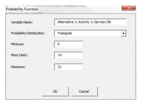
RealCost – Service Life for Initial Flexible Pavement Construction (Alternative 1: Activity 1)
