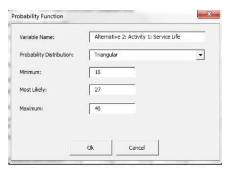
RealCost – Service Life for Initial Rigid Pavement Construction (Alternative 2: Activity 1)
